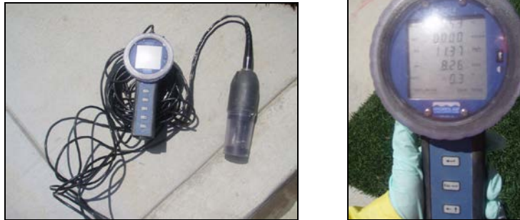
Figure D-2 Example of an All-In-One meter
